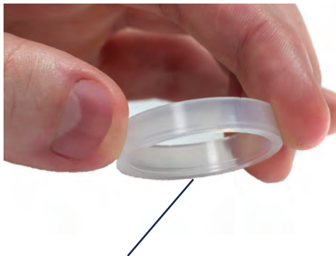
Flanged edge of the sample cup ring
